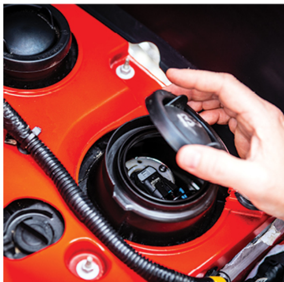
Tool-less headlight bulb replacement
