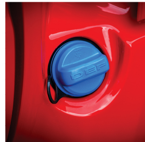
The DEF (Diesel Exhaust Fluid) tank fill point is located near the passenger side door to help avoid mixing the wrong fluids and allows the tank to be filled without opening the hood
